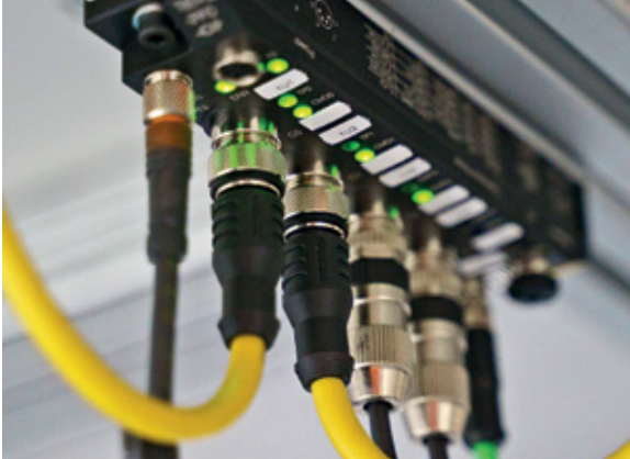
Turck's TBEN-S-RFID interface talks both Profinet with the Siemens PLC as well as Ethernet/IP as an interface to Labview on the rework station
