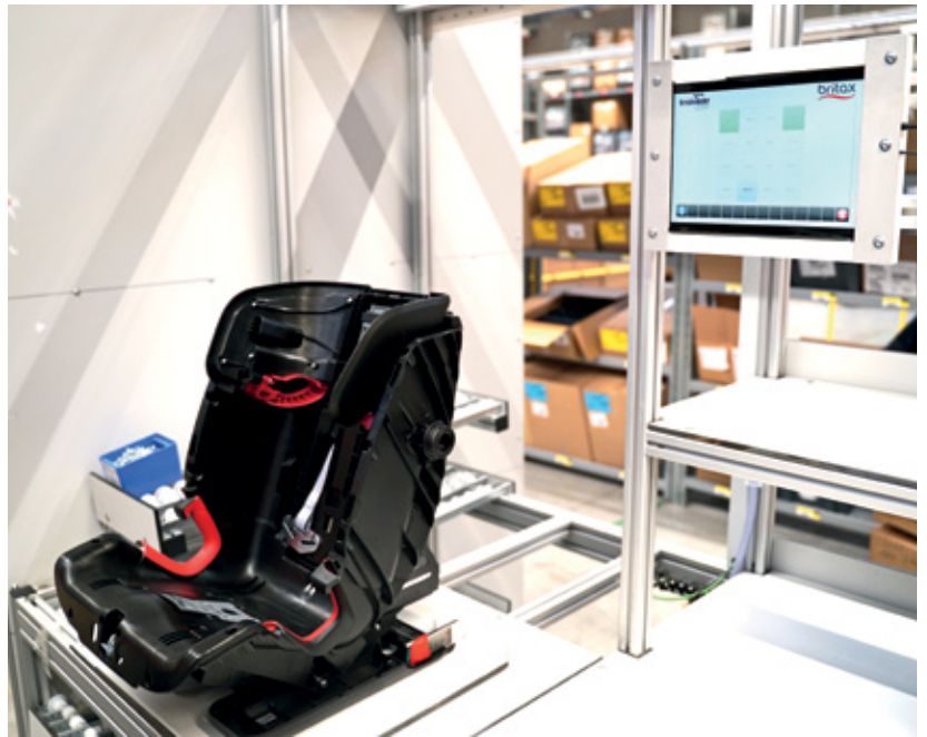
At a glance: The tablet (right) at the rework station shows via Labview which station has to be reworked
