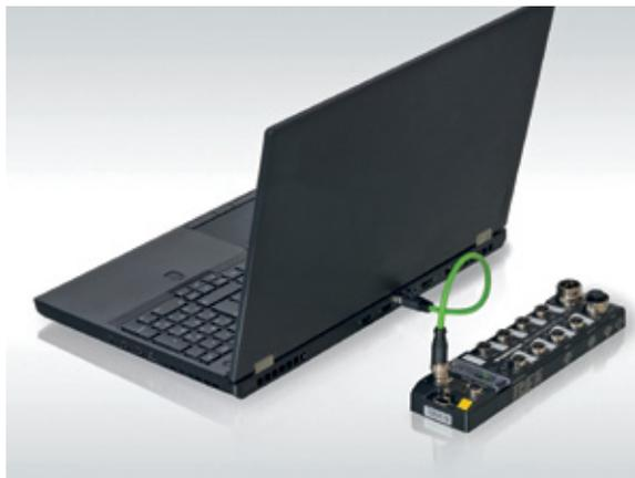
**New at the Hannover Messe: Turck's TBEN-L-RFID module with an integrated OPC UA server simplifies the connection of factory automation to the IT world**
