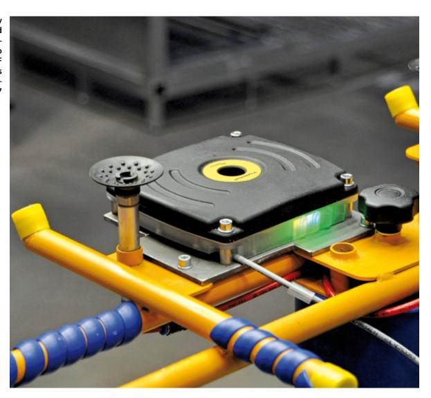
red and managed by the software. This allows tracking and tracing the bumpers during the entire production and logistical process. Prior to lacquering, the position of the bumper inside the skid is detected by a reader, and captured by the middleware. This is used to track the production quality. After the lacquering process the entire paint shop data is automatically linked to the bumper.
