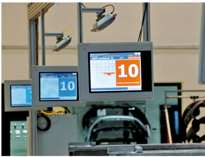
The UHF read/ write heads (above) monitor the storage of the bumpers in the containers
