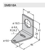
3033200 Mounting bracket, rectangular, stainless steel, for sensors with 18 mm thread
