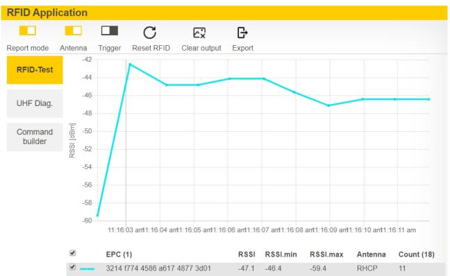
**RFID test** allows EPC information from tags to be displayed and read out in single-tag and multitag mode. The received RSSI values are displayed as a curve in relation to time.
