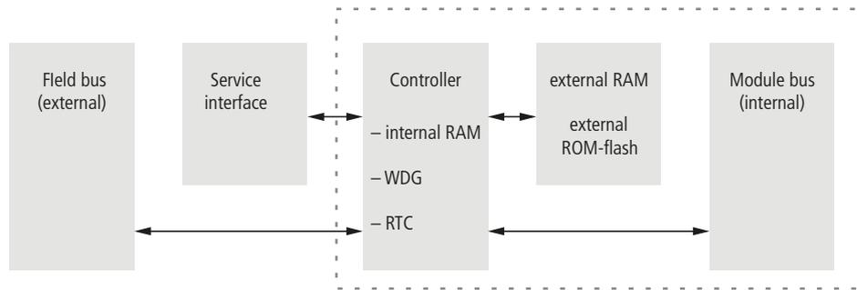
Fig.. 3: Structure of a BL20-E-GW-DP
