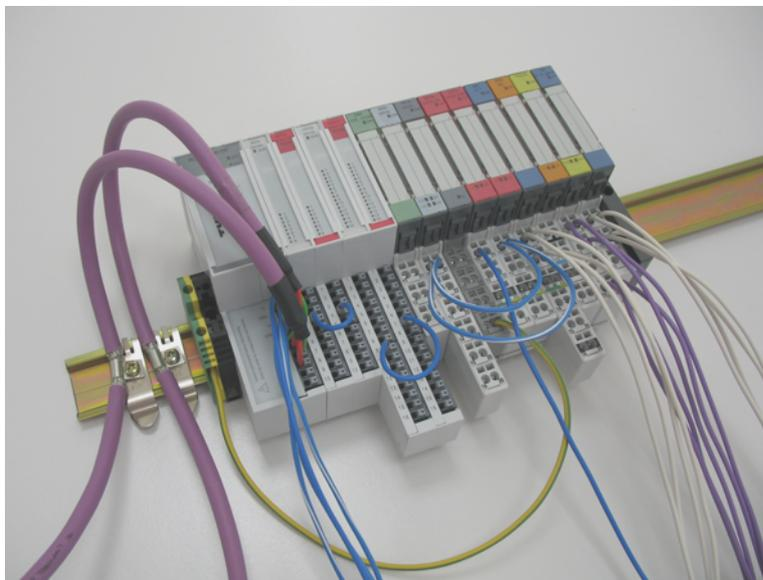
Fig. 23: Example of a station structure with ECO gateway, ECO and standard I/O modules
