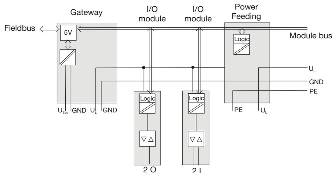
Fig. 29: Block diagram of a BL20 station with an ECO-DP gateway
