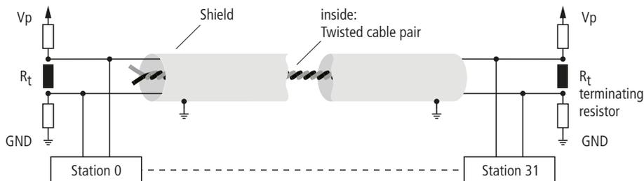
Fig. 28: Representation of a PROFIBUS-DP cable
