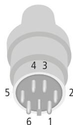
Fig.. 5: PS/2 plug on the connection cable to the gateway (top view)
