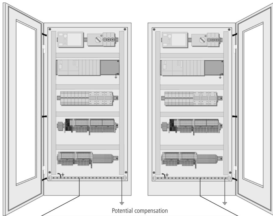
Fig. 32: Potential compensation between switchgear cabinets
