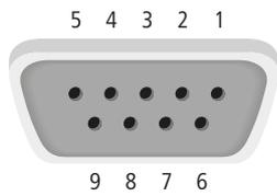
Fig.. 6: 9-pole SUB-D socket connector on the cable for connecting to PC (top view)
