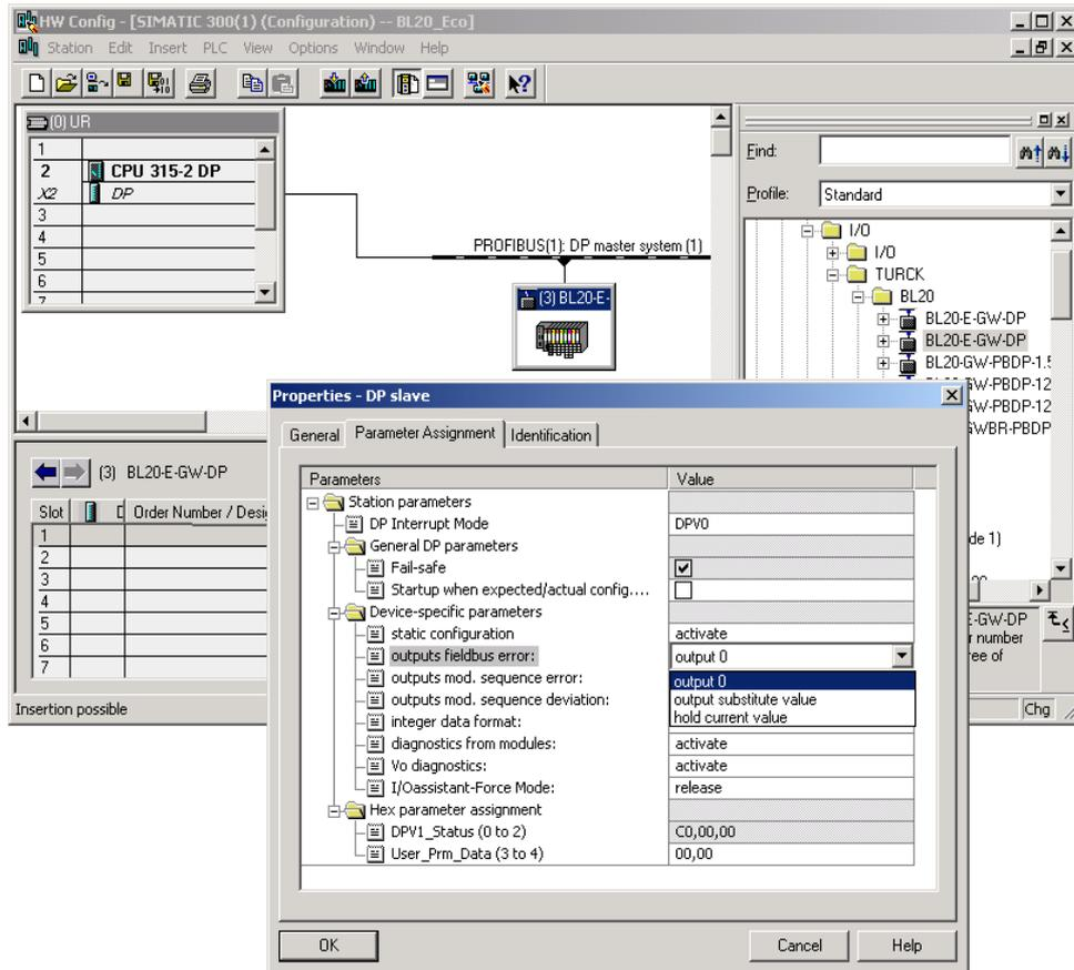
Fig. 13: Parameterization of the BL20-gateway
