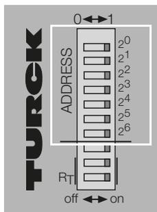
Fig.. 7: DIP-switches on the gateway
