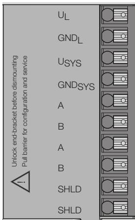
Fig.. 4: Push-in tension clamp terminals at the gateway
