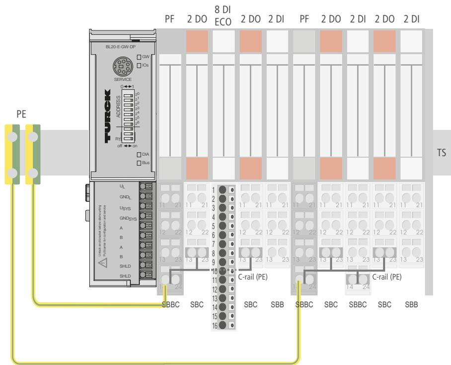
Fig. 26: Using the C-rail as a protective earth
