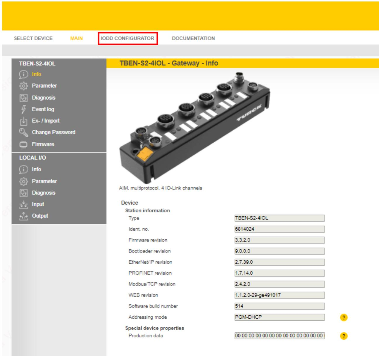
Fig. 31: Web server – IODD Configurator
