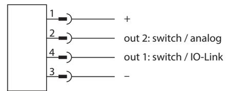
Fig. 18: LRS...LI2UPN wiring diagram
