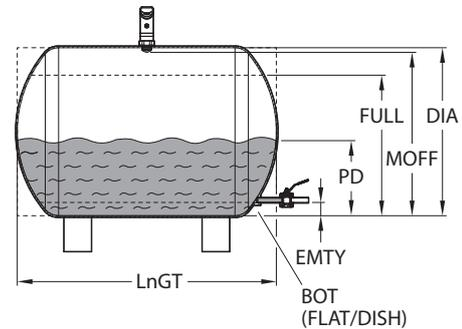
Fig. 28: Parameters – horizontal cylinder
