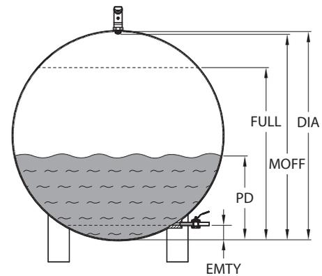
Fig. 30: Parameters – spherical container
