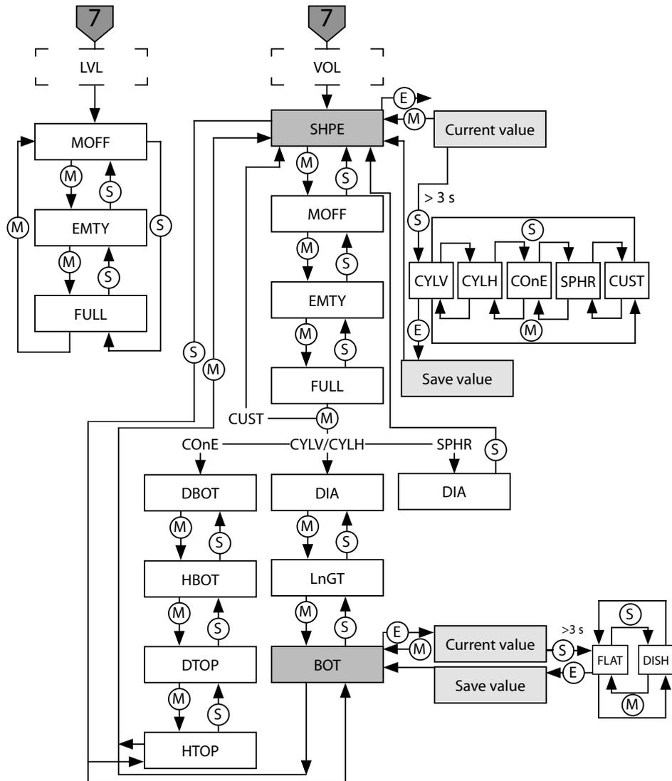
Fig. 26: Geometry submenu (GEOM)
