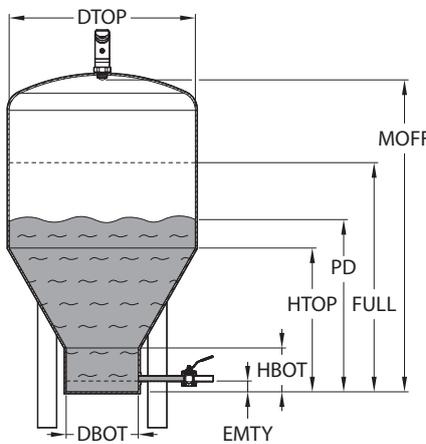
Fig. 29: Parameters – conical container
