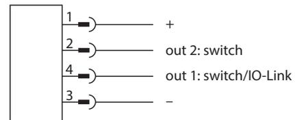
Fig. 20: LRS...2UPN... wiring diagram
