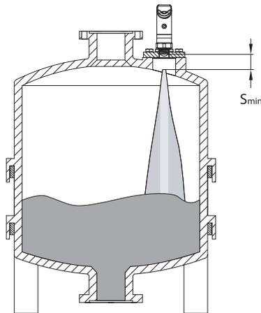
Fig. 14: Installing LRS510...
