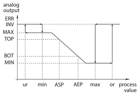
Fig. 13: Falling output characteristic, MIN = 0
