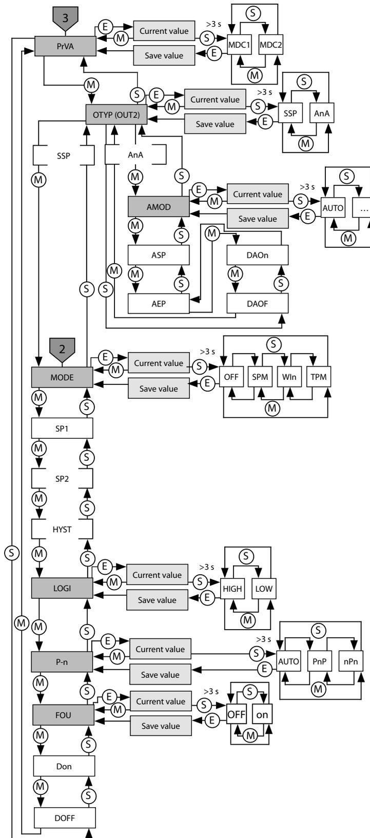
Fig. 24: Outputs submenu (OUT...)
