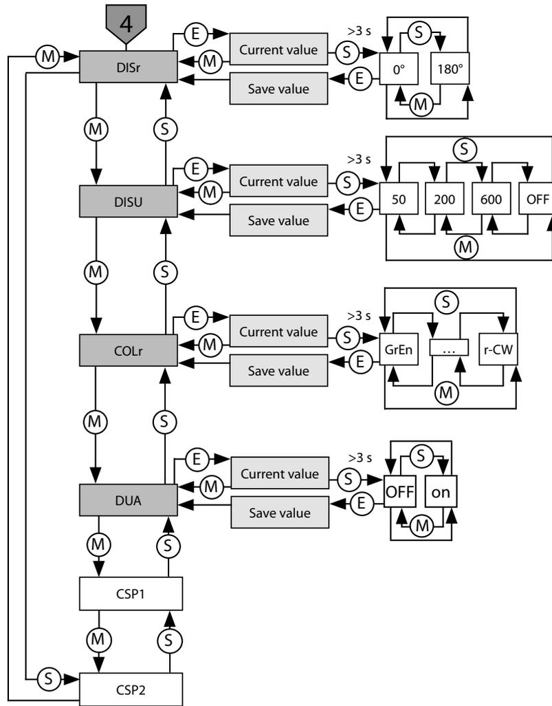
Fig. 25: Display submenu (DISP)
