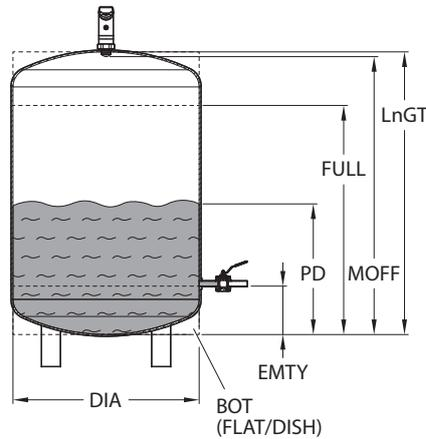
Fig. 27: Parameters – vertical cylinder
