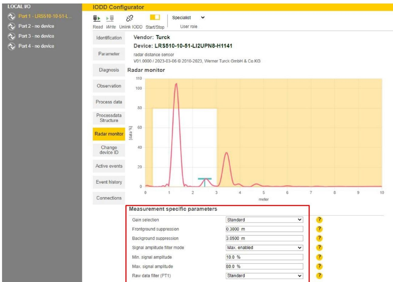
Fig. 34: Example – filtering signals
