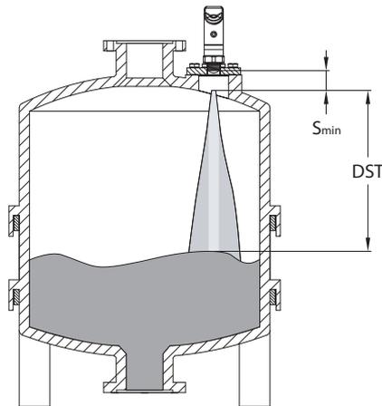
Fig. 6: Distance (DST) in containers
