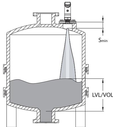
Fig. 7: Level (LVL) or container volume (VOL) in containers
