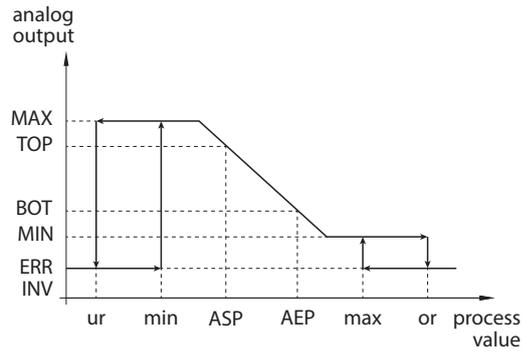
Fig. 12: Falling output characteristic, MIN  $\neq$  0
