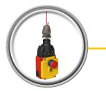
The safety rope pull switches of the RP-RM (metal housing) are approved for all commonly recognized standards. After actuation or in the event of a rope break, the E-stop device locks automatically and can only be reset by means of the reset feature on the device.
