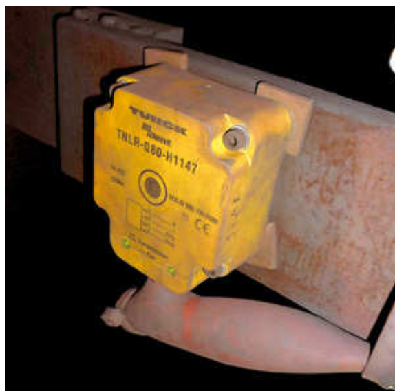
Turck's TNLR-Q80 read/write head didn't have any problems with the harsh environmental conditions
