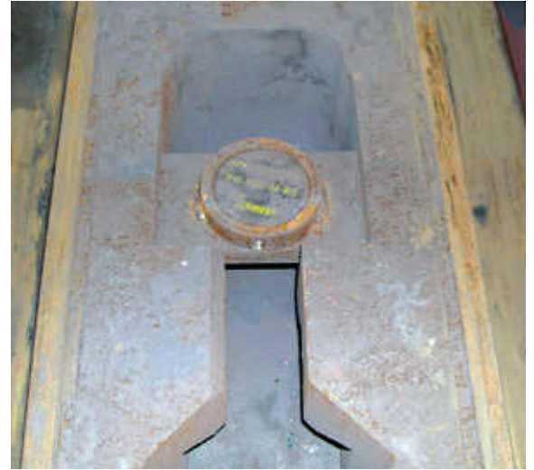
The tag is embedded in a steel ring and is nevertheless read reliably
