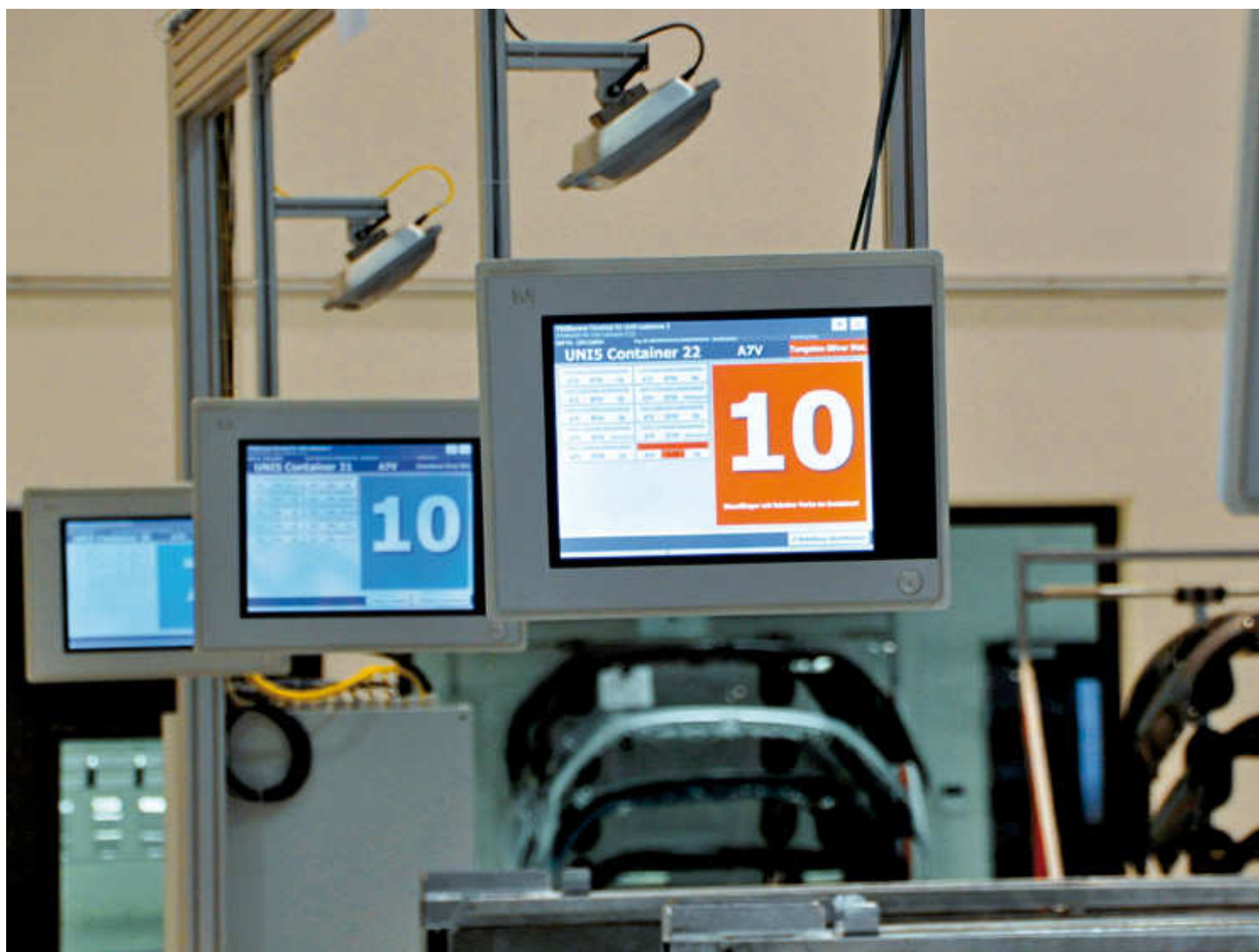
The UHF read/write heads (above) monitor the storage of the bumpers in the containers
