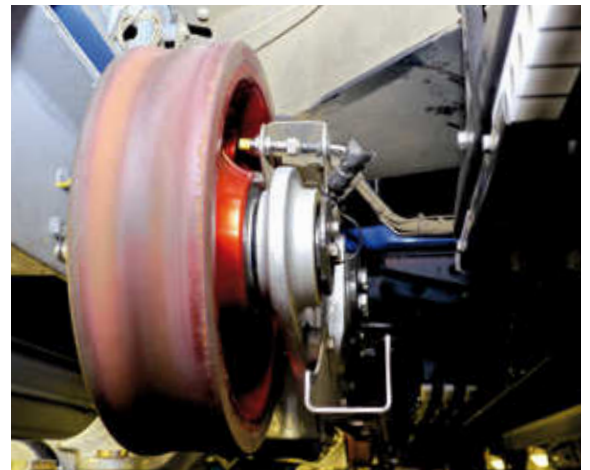
The hole in the alloy wheel of the Megacoaster is detected by the uprox+ with its precise switch point
