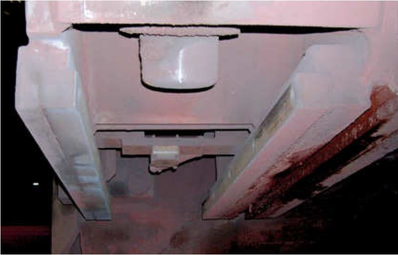
The cages are pushed into the rails of the rolling stand. The read/write head (center) identifies the tag on the rolling stand
