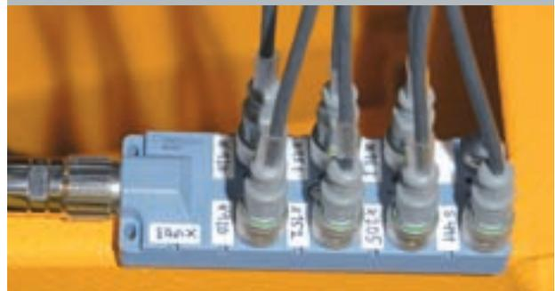
Turck boxes with rapid plug-in systems on Wumag’s aerial work platforms are extremely leakproof Page 32
